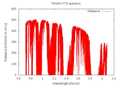
Radiance simulated by MARTA in a spectral region that covers the three SWIR bands measured by TANSO-FTS. In this simulation the instrumental effects have not been included.
